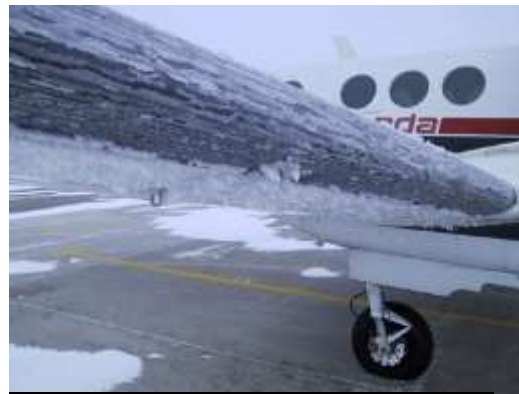
Mixed ice is a combination of rime and clear ice. Ice can distort the flow of air over the wing, diminishing the wing's maximum lift, reducing the angle of attack for maximum lift, adversely affecting airplane handling qualities, and significantly increasing drag.
