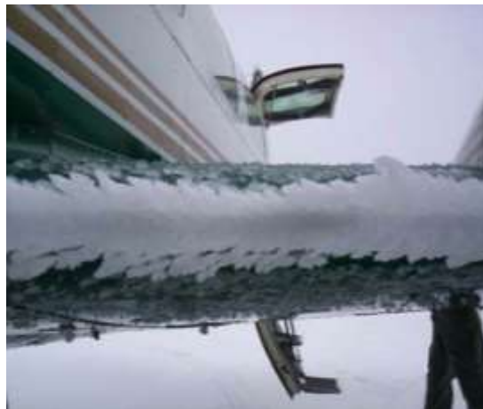
Rime ice has a rough, milky white appearance, and generally follows the contours of the surface closely. Much of it can be removed by deice systems or prevented by anti-ice
