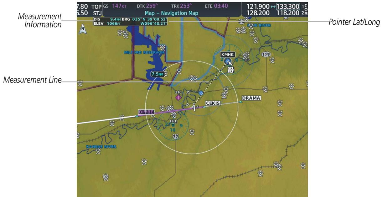
Figure 5-11 Navigation Map - Measuring Bearing and Distance
