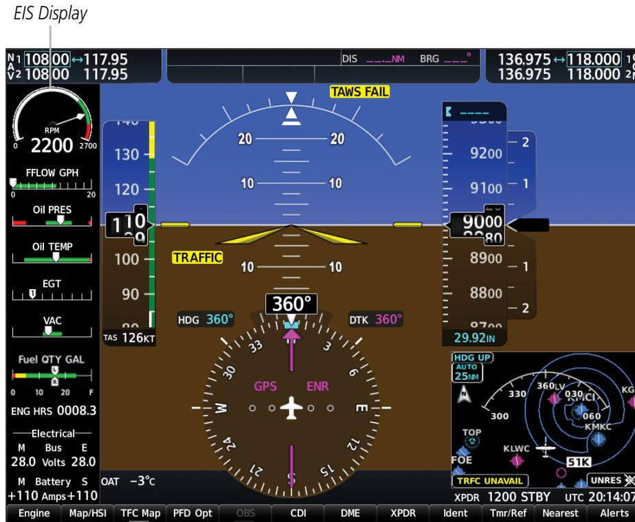
Figure 3-18 Reversionary Mode (EIS Shown)
