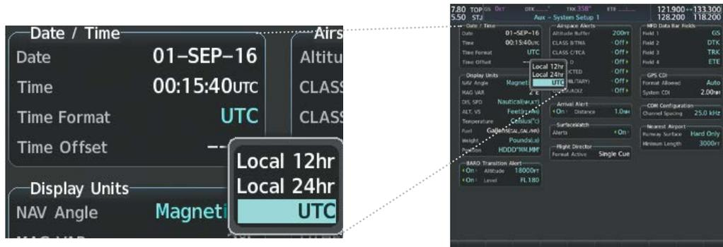
Figure 1-14 Date/Time Settings (System Setup 1 Page)
