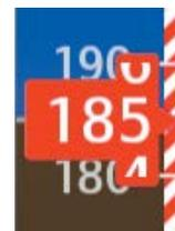
Figure 2-4 Red Pointer Showing Airspeed Above  $V_{NE}$
