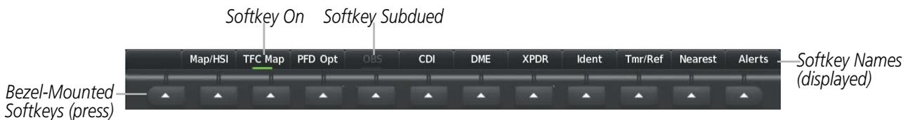
Figure 1-9 Softkeys (First-Level PFD Configuration)
