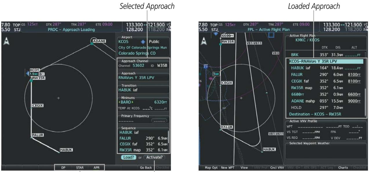
Procedure Loading Page Selection Softkeys LOAD or ACTIVATE? Annunciation
