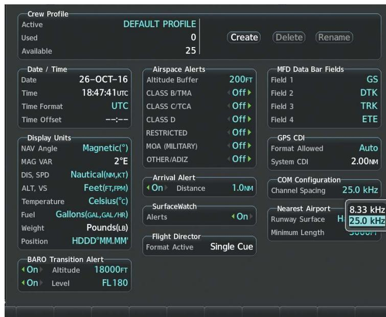
Select 8.33-kHz or 25.0-kHz COM Frequency Channel Spacing
