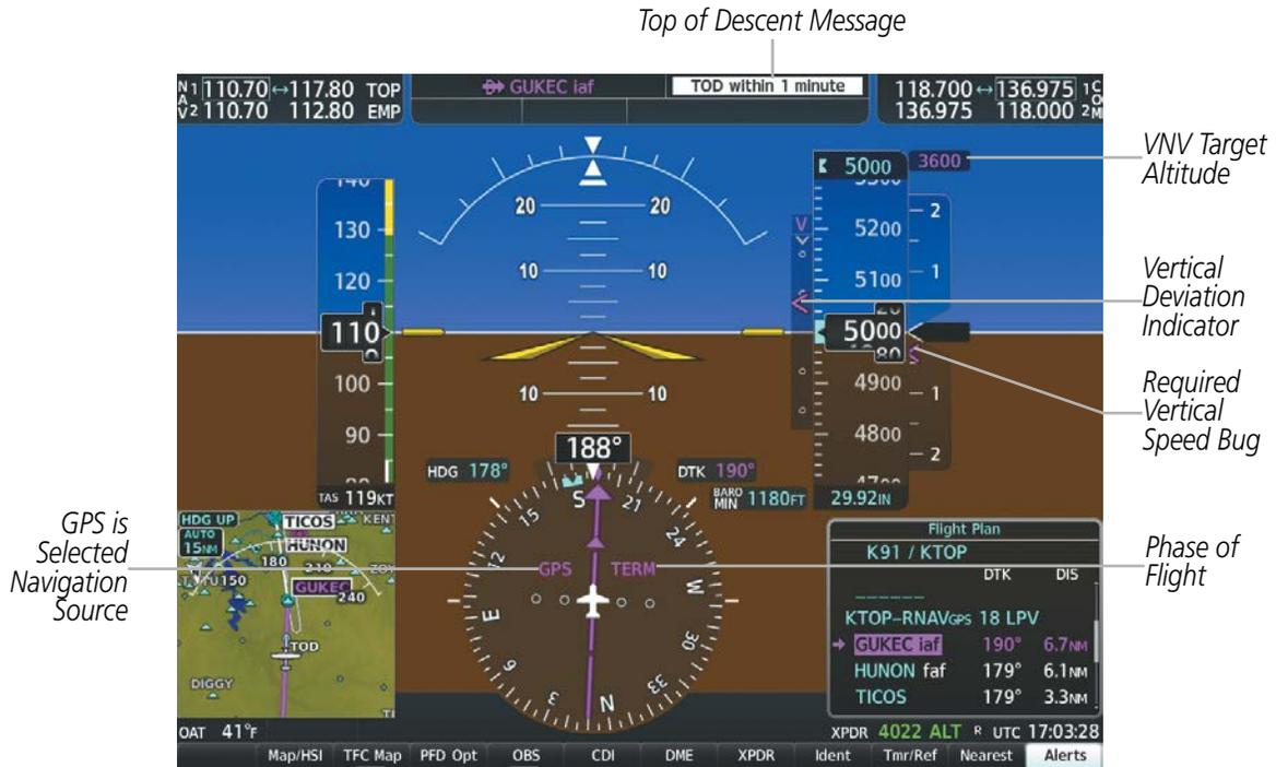
Figure 2-30 Vertical Navigation Indications (PFD)
