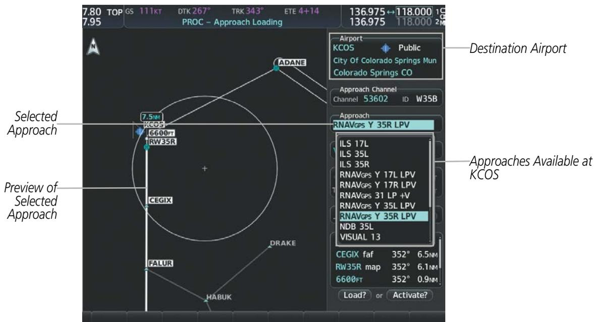
Figure 5-60 Approach Loading Page - Selecting the Approach
