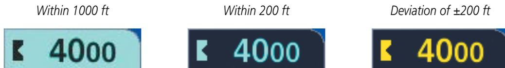
Figure 2-32 Altitude Alerting Visual Annunciations
