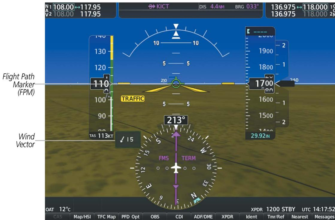
**Figure 8-6 Flight Path Marker and Pathways**
