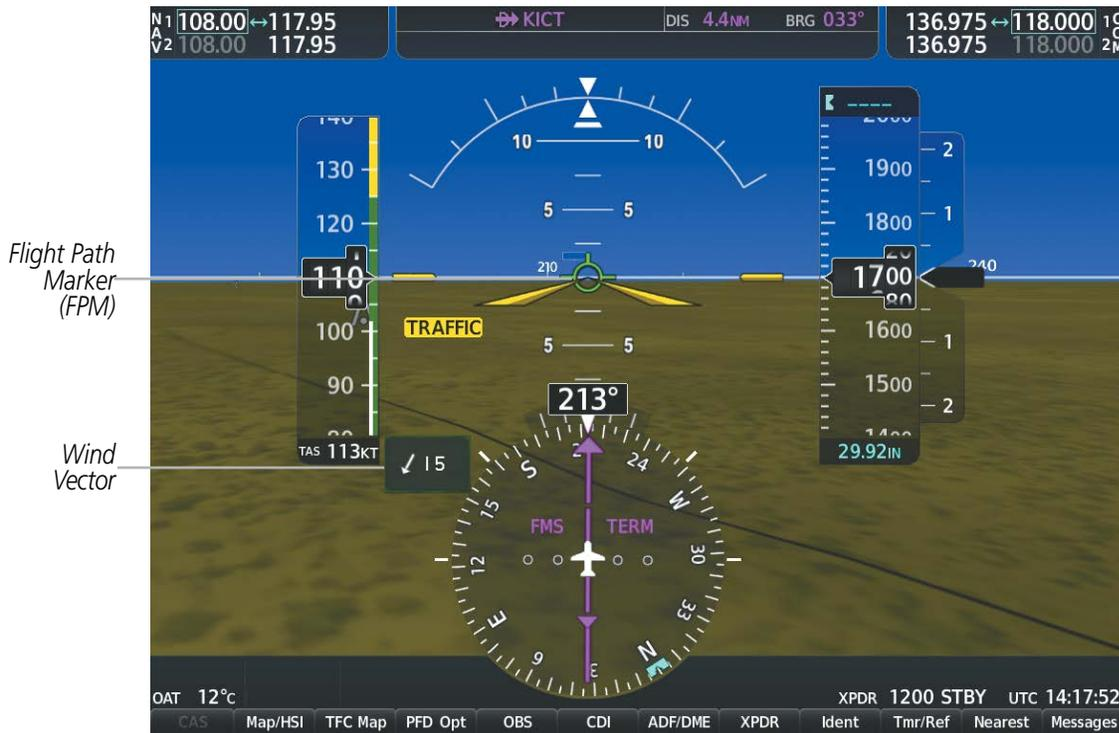
**Figure 8-6 Flight Path Marker and Pathways**
