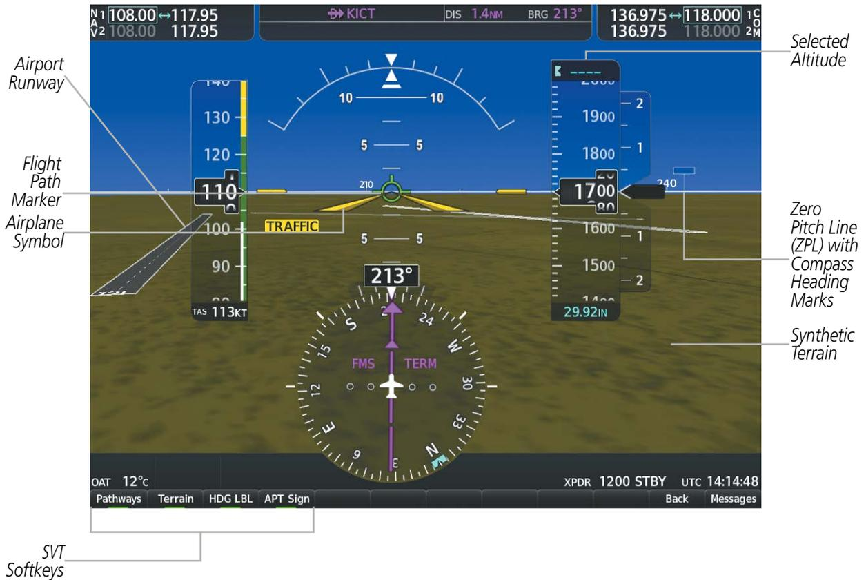
Figure 8-2 SVT on the Primary Flight Display
