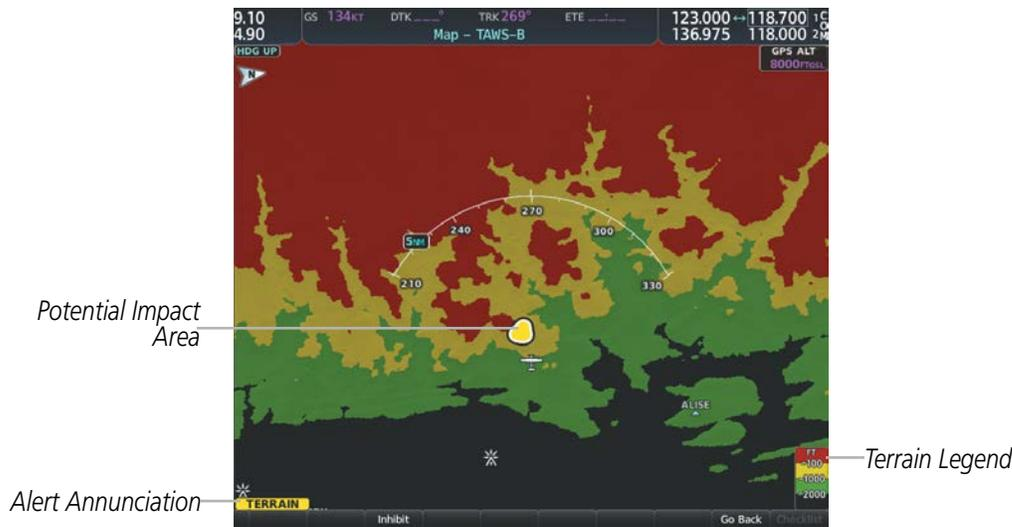
Figure 6-59 Navigation Map Page (After TAWS-B Pop-up Alert Acknowledgment)
