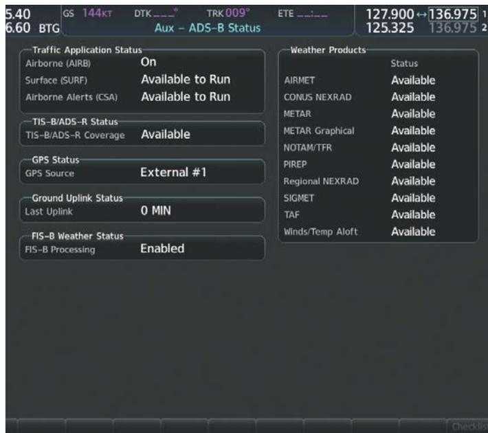
Figure 6-79 Viewing ADS-B Traffic Status on ADS-B Status Page
