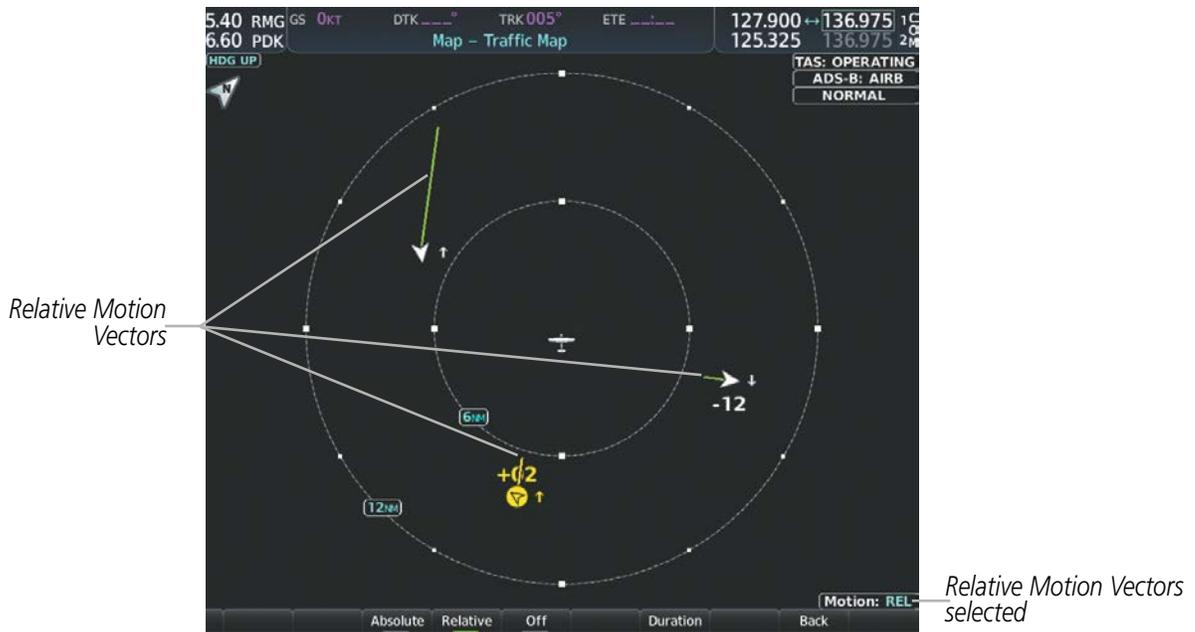
Figure 6-78 Traffic Map Page with Relative Motion Vectors Enabled
